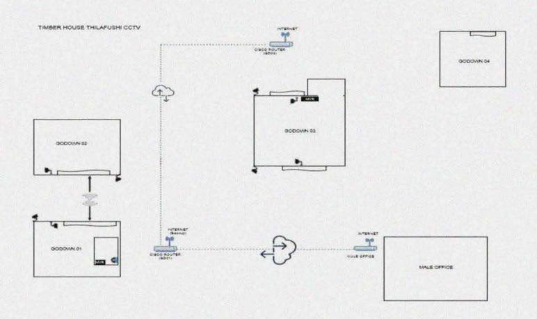
SAFE NETWORK Proposes an CCTV monitoring solution that can monitor environment and Backup Footage. Solution propose to install a 3 Major Location along with Local Footage Backup and Optional CCTV Monitoring through Internet
